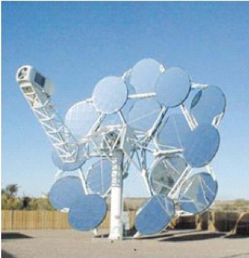
This Science Application International Corporation/ STM Power Inc. 25 kW Dish-Stirling System is operating at a Salt River Project site in Phoenix, AZ.
